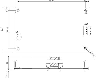
DC Input Connector (CN1): JST B3P-VH-B or equivalent
