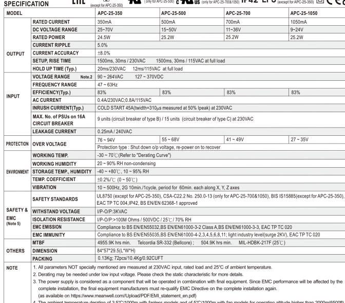
The ambient temperature derating of 3.5°C/1000m with fanless models and of 5°C/1000m with fan models for operating altitude higher than 2000m(6500ft).
