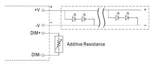
"DO NOT connect "DIM- to -V"
