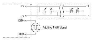
"DO NOT connect "DIM- to -V"
