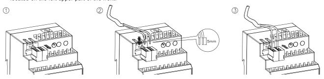
c. Connect the mains voltage, the connection to the AC is made with the terminal (L, N,  $\stackrel{\perp}{=}$  ) located on the bottom.
