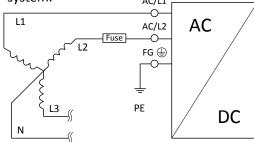
Using a fuse or a circuit break to protect the AC/L2 input is suggested. The AC/L2 input is internally non-protected. Suggested fuse is shown as below.
