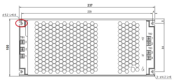
The mounting hole circled in red is the protective ground. Please use M5 screw with the diameter of the screw head less than 8mm.
