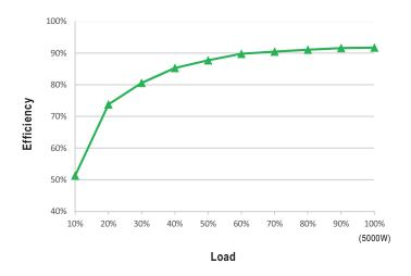
Energy recycling ratio = Efficiency 1 (power supply) x Efficiency 2 (ERG-5000 series)
