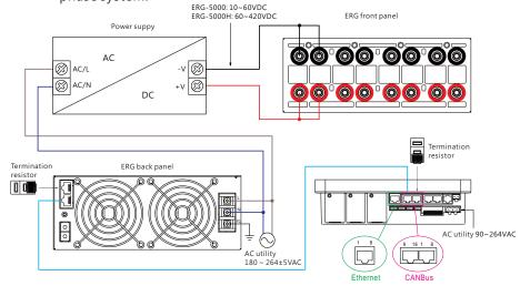
NOTE: After connecting the communication cable, install termination resistors to the remaining sockets of both the ERG-5000 series and CMU2A to prevent signal reflections.
