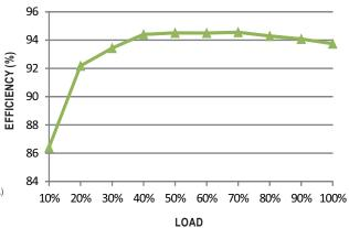
The curve above is measured at 230VAC.
