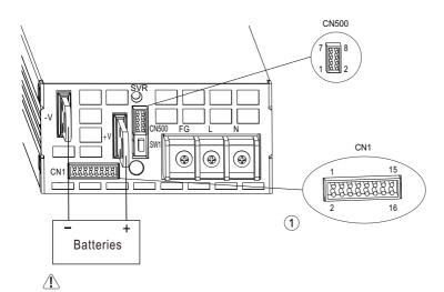
Warning: Before connecting a battery, please make sure the polarity is correct to avoid damaging the charger
